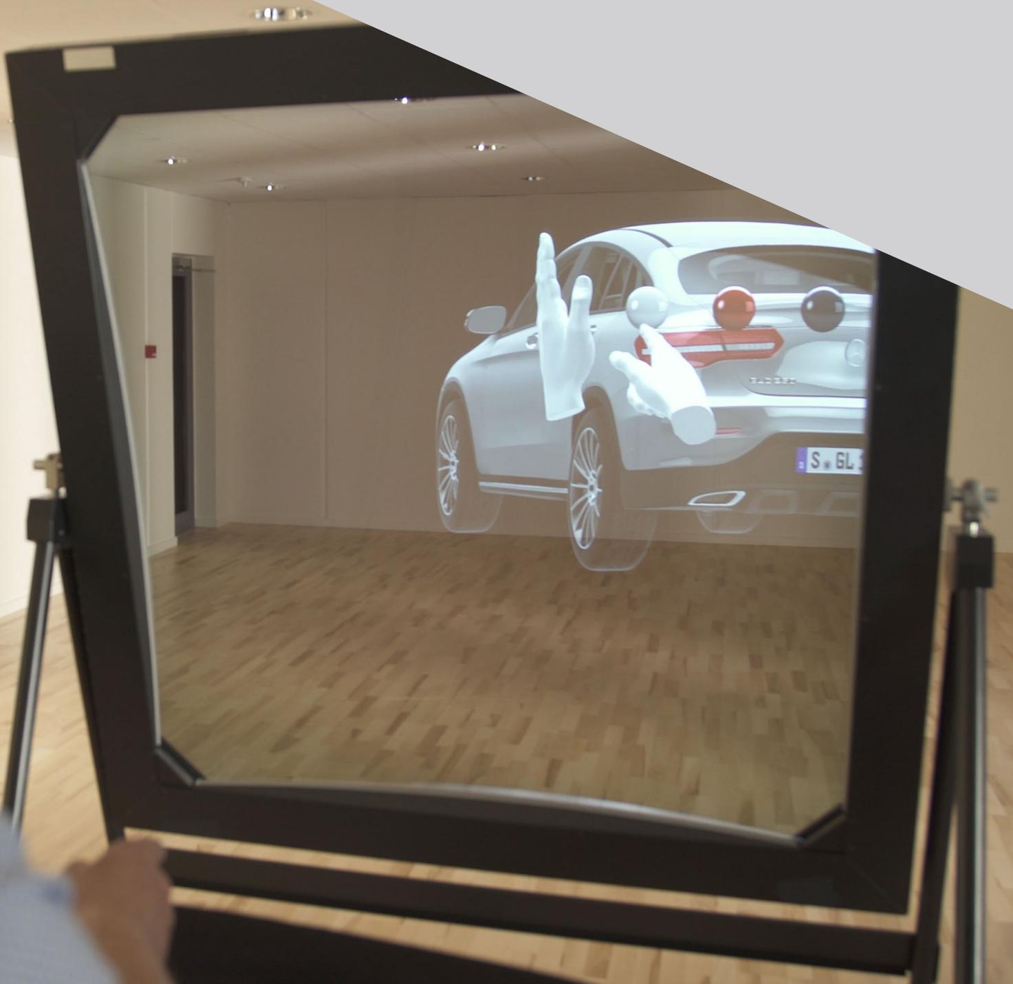
DeepFrame is a revolutionary new type of mixed reality display that enables digital content to appear as a hologram on top of reality seen through the lens. The window-like display consists of a high-precision optical lens that can be mounted on the floor stand (optional accessory) or hang suspended in wires.
