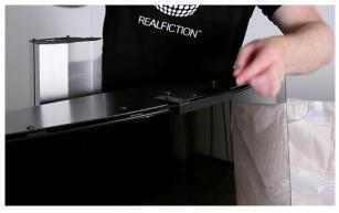
7. Take the Connection Cable and mount it to the Sound Bar. Fasten with the 2 small black screws.
