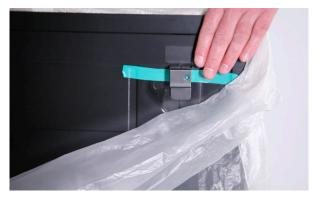
3. Lift the OLED Screen in place, one side at a time, by hinging the bracket to the OLED Mount.
