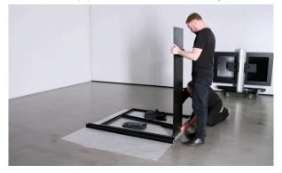
3. Attach one of the black aluminum profiles to the side frame and lock it in place using an umbraco key.
