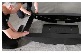
6. Take the Vesa Mount Holder and place it in the middle of the OLED Mount with the flat side facing upwards. Attach it with 4 screws each for the top and bottom. When all the screws are fitted, make sure to tighten them completely.
