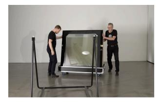
6. Gently lift out the Optical Lens Optic and rest in on a sheet of protective foam on the floor.
