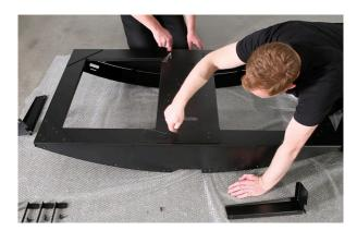
7. Raise the OLED Mount Kit upwards and the attach the stabilizer inside, with the flat side towards you. Attach it with 1 screw for the top and bottom.
