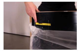
12. Lift the OLED Screen in place, one side at a time, by hinging the bracket to the OLED Mount.
