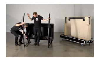
8. Take out the Optic Safety Bracket and slide it down into the holes on the top of each Leg Frame, as this will set the correct distance between the leg structures and provide support when mounting the DeepFrame Optical Lens afterwards.
