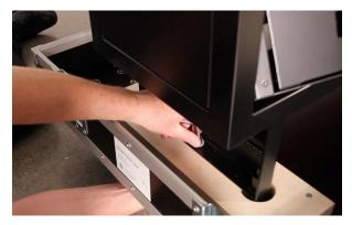
5. When the bolts have been removed, lift the OLED Housing out from the flight case and place it on the floor.
