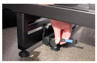
4. Use the search spring from the Toolbox and guide it through the small hole in the Leg Frame located under the Speaker Module, until it comes out of the hole where you removed the plastic plug.
