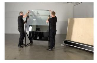
10. Secure the DeepFrame Optical Lens in place using 1 long black 10mm bolt in each side – make sure you do not use the transport bolts you have removed previously.
