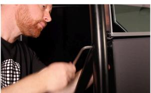
3. In one side of the Speaker Module you will see the speaker cable. The next step is to guide this cable through the Leg Frame. Under the DeepFrame Housing, locate the 2 plastic plugs in the Leg Frame and remove the left one.
