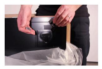
11. On the backside of the OLED Screen, guide the bracket through the bottom of the T-hole first and then slide it up and out towards the corner of the screen. Secure it in place using a piece of tape. Repeat this for the other side as well.
