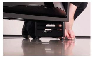
7. In the other flight case, take out the first Leg Frame and attach it with 2 bolts in the lowest of the grooves underneath the OLED Housing, using spanner size 19. Then, take out the second Leg Frame and attach it in the same way.
