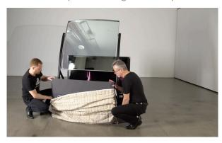
2. Gently lift it over to the Leg Frames underneath the DeepFrame Optical Lens and attach the lower part first by sliding the notches in to fit the pins on each Leg Frame. Then slowly raise it upwards and fasten with 1 long black 10mm bolt in each side.
