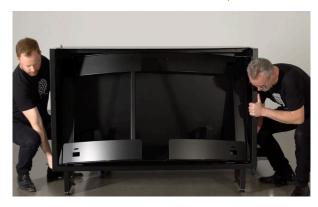
6. Place the spirit level on top and adjust the feet using a spanner size 13 until the OLED Housing is correctly levelled.
