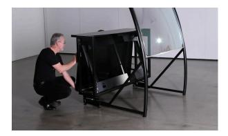
4. Loosen the screw for the Screen Adjuster located in each side.
