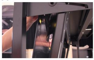
13. Then very gently hinge the other side on, thereby curving the OLED Screen to fit the OLED Mount. Important: Do not apply pressure to the bottom part of the OLED Screen, instead allow the bottom corner to bend in a different radius than the top, leaving a wider gap!
