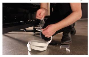
2. Attach the Black Cable Lock to the Connection Cable Extender and mount it to the Sound Bar. Fasten with the 2 small black screws.
