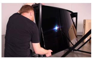
14. When both sides are hinged in place, guide the screws through the holes and fasten with the wing nuts and washers to secure it in place, one side at a time.
