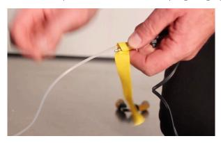
6. Connect the speaker cable to the Sound Bar (Speaker Out, Stereo (8 Ohm)).
