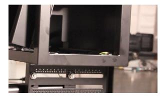
8. Lastly, attach the 2 side plates, the front plate and the plates in the bottom on the OLED Housing again.
