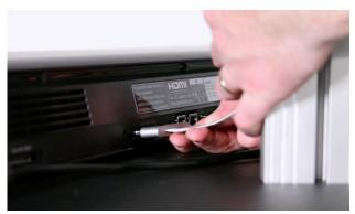
6. Insert the Connection Cable to the Sound Bar and then connect it to a power outlet.
