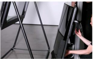
4. Then gently open the locks on the Optical Lens frame and rotate it to adjust the height your hologram appears in. When the right position is found, tighten the locks again to secure it in place.
