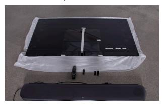
2. Remove all the protective foil from the backside of the OLED Screen. Also take off the white cuff that protects the Connection Cable in order to remove the protective foil in that area as well.
