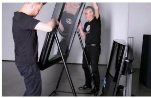
4. Finally, tilt the OLED Screen to obtain the same angle as the Optical Lens. This step is to eliminate distortions in the hologram.
