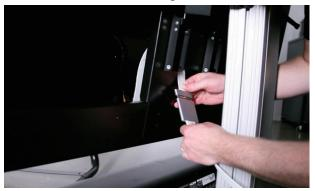
2. We always recommend placing the OLED screen as high on the OLED stand, as this will limit the line distortion as much as possible.
