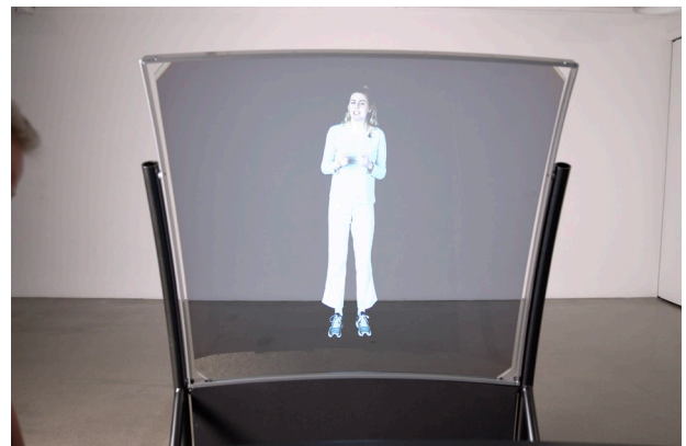
Screen furthest away from the Optical lens = the hologram is big
