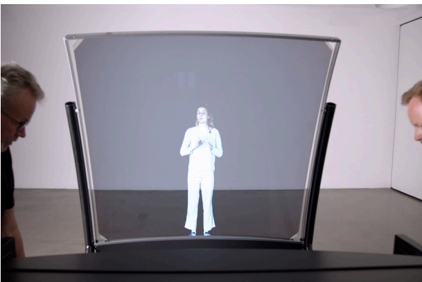
Screen closest to the Optical lens = the hologram is small
