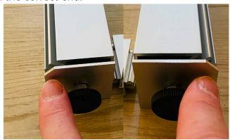
**3.** When connecting the aluminum profiles, make sure that the groove on the cross profiles align perfectly with the groove in the corner profile. Tighten the screws to lock the profiles together.
