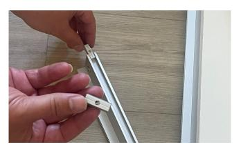
**2.** Attach the black bracket to the two nuts with two screws. Position the bracket at the center of the profile before tightening the screws. Attach the cross profile to the stand again.
