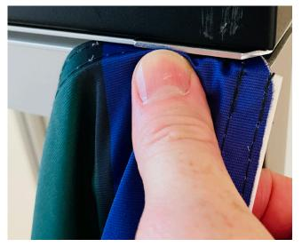
**2.** Continue to push the thick edge of the print inside the groove all the way around the edge. When mounted correctly the print will stretch neatly and leave a smooth surface.
