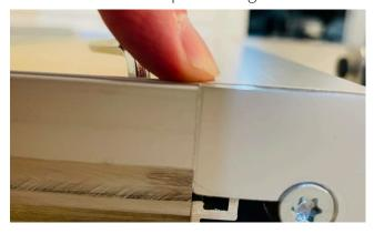
**4.** When all 4 profiles are securely locked together, turn the frame around, so the slanted corners are now facing towards the floor. Then attach the 4 short cross profiles - again making sure the TOP variants and BOTTOM variants are correctly positioned, and that the outer grooves are perfectly aligned.
