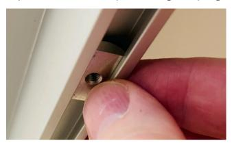
**2.** Next, push a safety bracket into the groove in the black plastic profile in the bottom of the display, and then adjust the position of the bracket and the spring nut, so the holes align perfectly.
