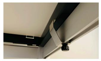
**1.** First insert the spring nuts - one in each side - in the groove in the stand underneath the display. Press one side of the nut up in the groove first, and then push the other side up, activating the spring.
