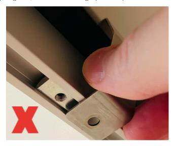
**3.** Fix the brackets with the two finger screws. The display is now fixed to the stand.
