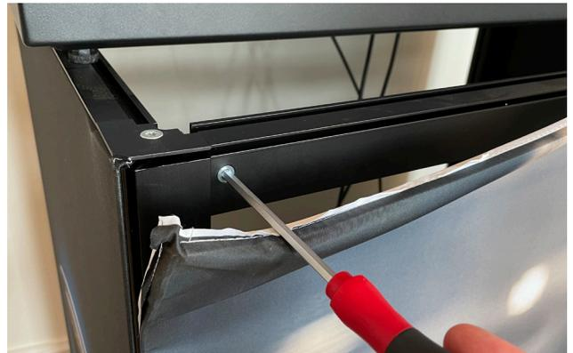
Start by loosening one side of the front topbar on the stand using a 5 mm unbraco key. The screw is hidden behind the cloth. Be careful only to loosen the screw. Do not remove it!
