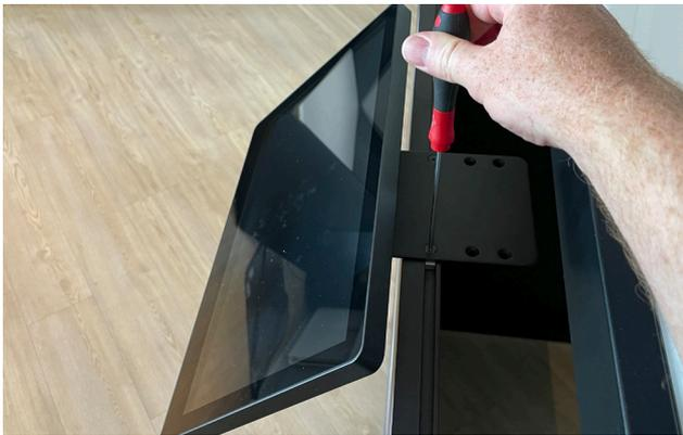
Attach the vesa mount to the silver brackets, using two countersunk hexagon socket screws and a 2 mm unbraco key.
