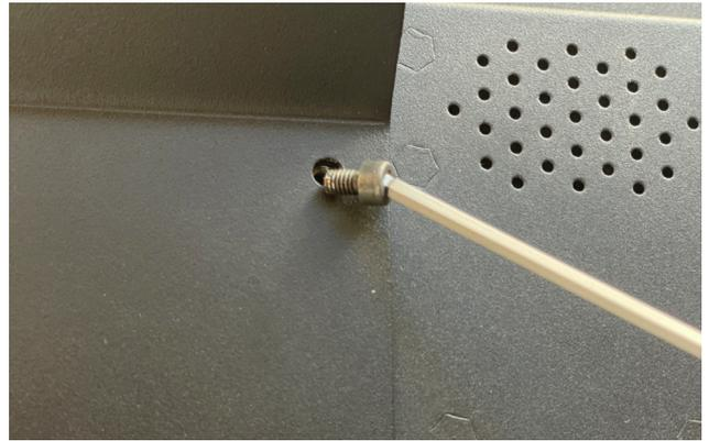
This is done with 4 cap hexagon socket screws that come with the vesa mount and a 2 mm unbraco key. Do not overtighten the screws!
