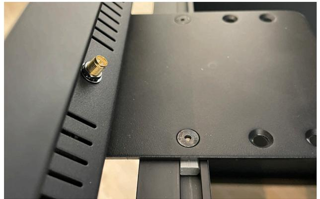
Before firmly tightening the two screws, you can adjust the exact position of the touchscreen.
