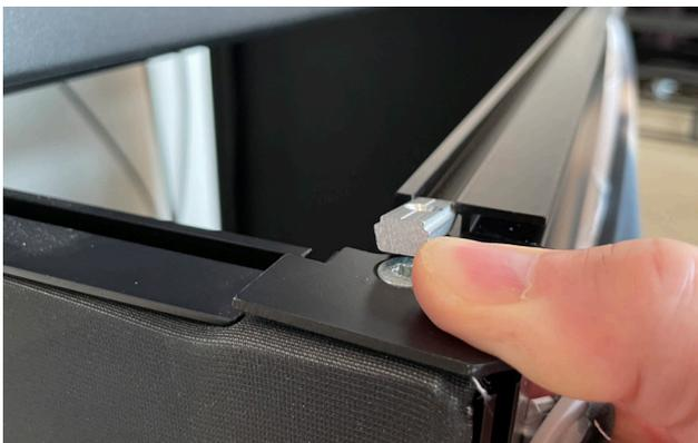
With one side loose, you can push the bar up just enough to slide the two silver brackets that comes with the vesa mount into the groove on the bar.
