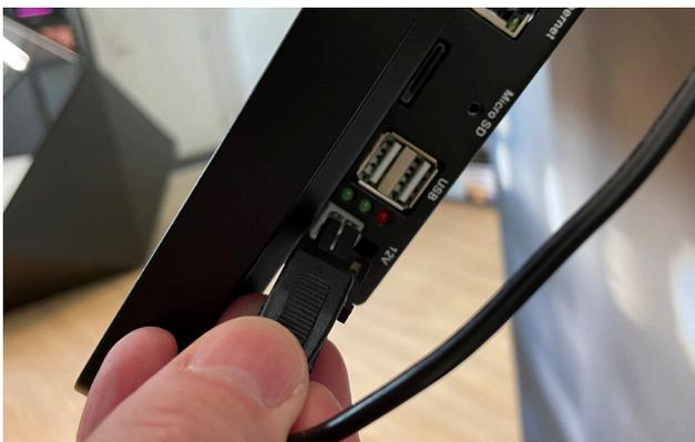
Connect the cable from the power supply to the right side of the touchscreen.
