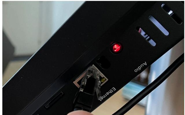
Insert the cable in the slot on the right side of the touchscreen.
