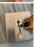
Unscrew the 2 screws shown here to remove the lamp shade
