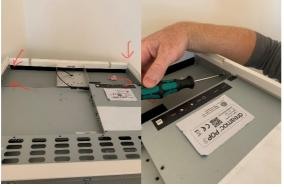
4. Unscrew the 4 screws that holds the metal plate. Be sure to have one hand holding the metal plate to prevent this from falling down when being loose.
