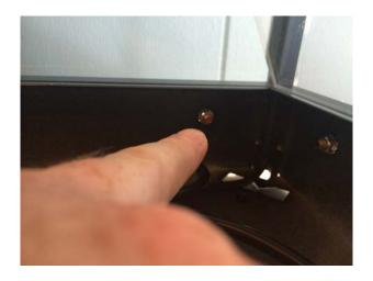
7) Important: When remounting the side plates, make sure note to over-tighten the nuts, as you might damage the aluminum and create bumps on the outside surface. Preferably use a machine with the screw torque setting **5**.
