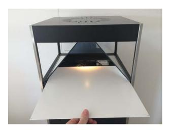
6) All 3 side plates should now be removed. Each side plate is fixed with 2 M5 self locking nuts from the inside. When you remove those 2 nuts, the side plate can be easily be removed, and that side optic can be removed as well.
