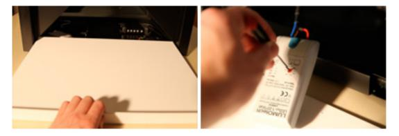
The Dreamoc also comes with a preinstalled light mask that focuses the light in a smaller area inside the Dreamoc, and reduce the brightness of the lamp slightly. This light mask can be easily removed by pulling it down gently with a finger inside the mask.
