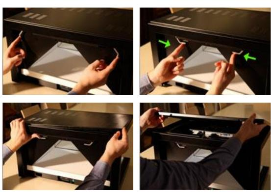
**Step 4.**Remove the power cable and the HDMI cable from the LCD screen and then remove the LCD screen from the Dreamoc HD.
