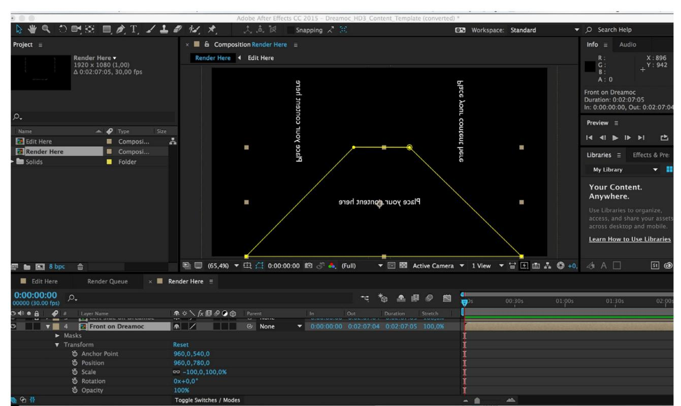
The second composition is called "Render Here". In this comp we have placed the comp "Edit Here" 3 times for front, left and right. They have all been mirrored, and each one is then rotated and positioned to fit the 3 sides of the display. See details of the front here.
