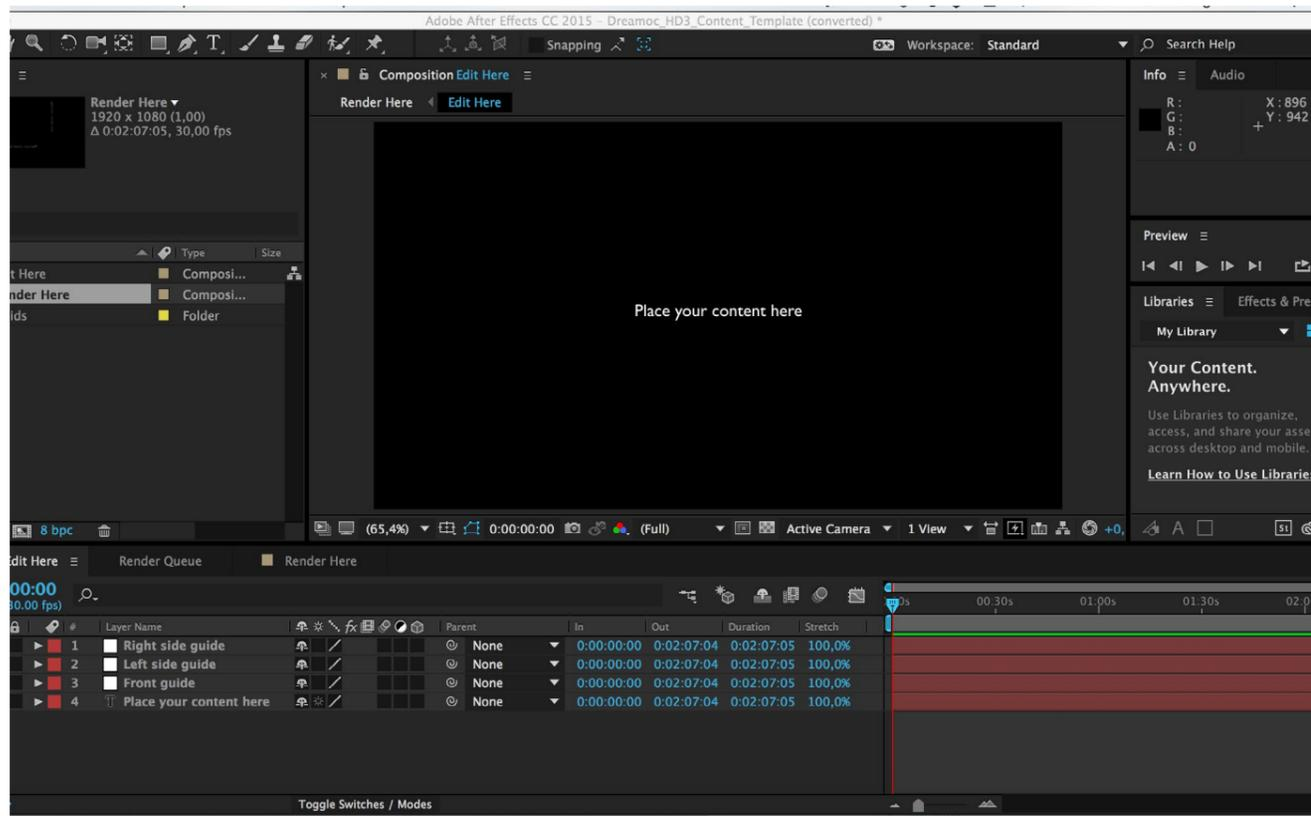
The Dreamoc HD3 template consists of 2 compositions. The first one is called "Edit Here". The idea is that you place your animation in this comp, and scale it to fit the HD3 format, by using the 3 guide layers. The composition is 1920x1080, square pixels.
