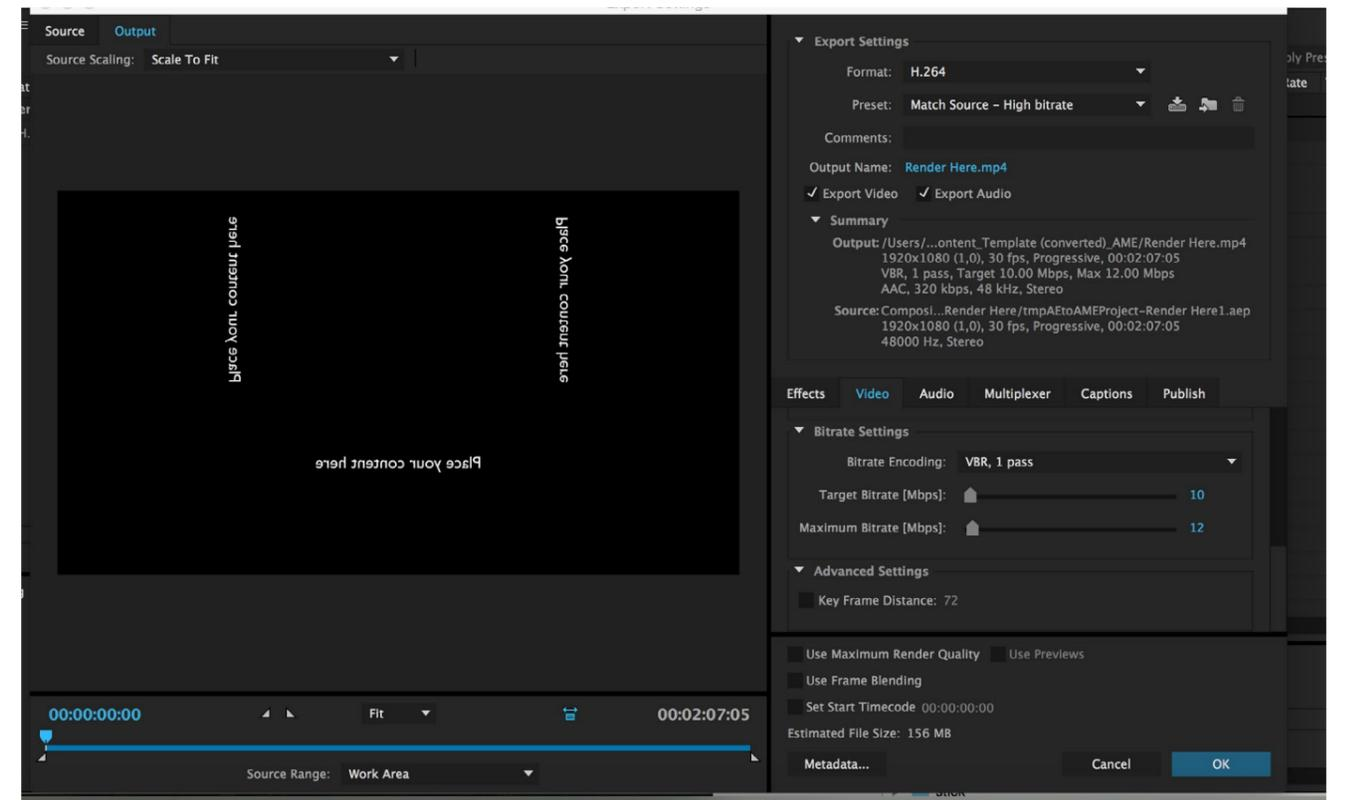
Finally this is an example of render settings used for the HD3. Many formats can be used, so this is just a suggestion. We use Mac, and render in MP4, with a bitrate of 10-12 Mbps.
