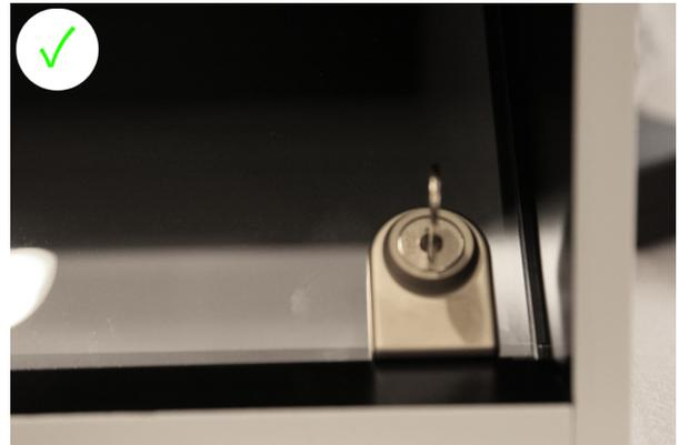
Lift up the optic by hand with the cleaning cloth and with your other hand place the object inside the display. When you are done gently slide back the optic and secure the lock.
