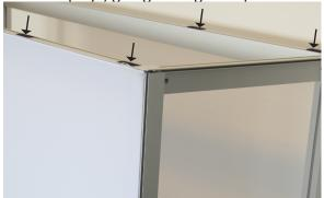
5. Mount the stand print on each side by pressing the silicone seam the into the external groove of the aluminum profiles. Begin with the four corners, and then press in the remaining parts. This method secures a tight and even fit to the stand frame.
