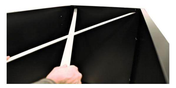
Once the brace is in place, grab a wing screw and screw it onto the bolts sticking down as showed below.
