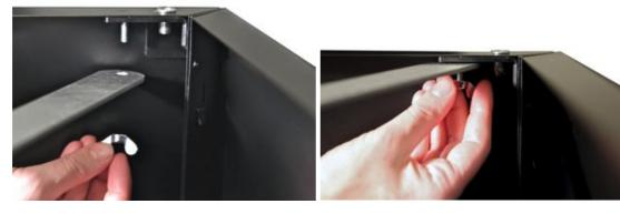
(5) Now the structure is assembled, and the feet should be attached. In every corner there is a hole for screwing the feet on. Grab the four feet and screw them on as showed below.
